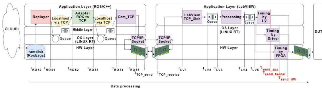
Figure 1: Detailed Conceptual Model and Software (SW) Instrumentation.
