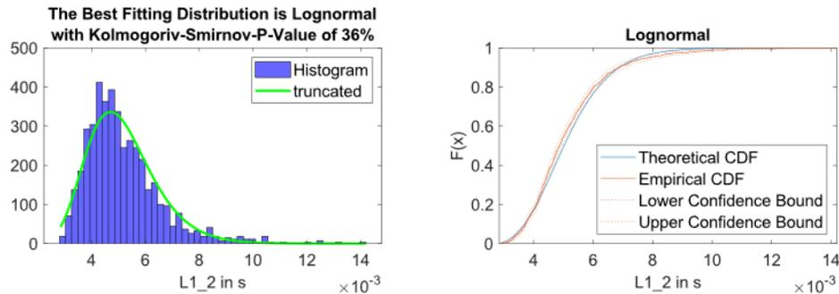
Figure 3: from left to right: Histogram and Distribution Fit of ROS Process Latencies, Comparison between Theoretical & Empirical Cumulative Distribution Function (CDF).
