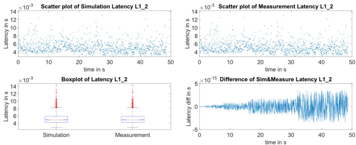
Figure 2: Example of process service times; from left to right: upper figures: scatter plot of simulation and measurement data, lower figures: Boxplot of Simulation and Measurements, Difference between Simulation and Measurements at each point over time.
