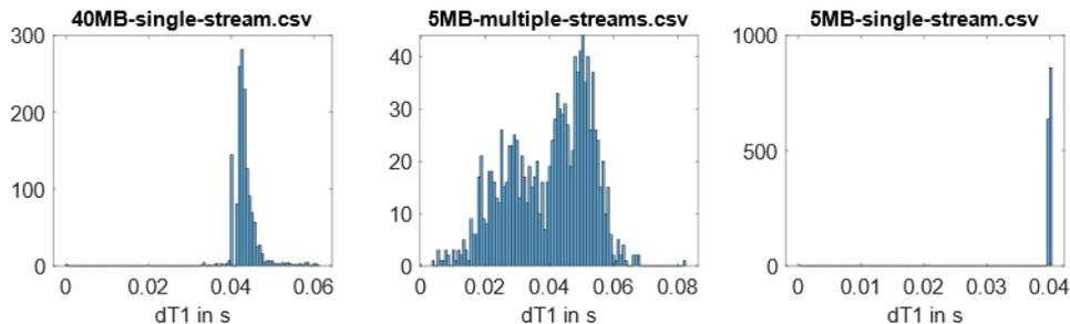
Figure 4: Histogram plots of 40ms cycle-time measured stream; from left to right: 40MB single stream; 5MB stream with 16 other streams in parallel, 5MB single stream.
