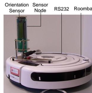
Figure 4: Roomba with mounted Sensor Node
