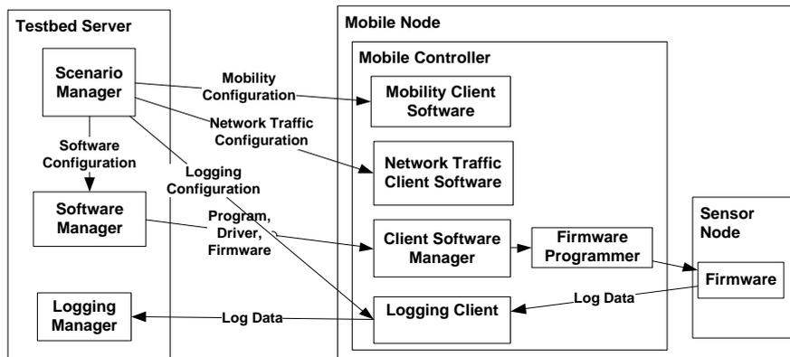
Figure 2: Interaction of Functional Blocks (Software)
