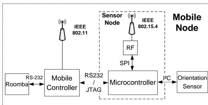
Figure 3: Block Diagram of Mobile Node
