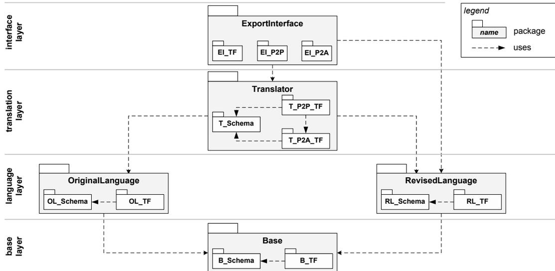
Figure 4: Package structure of the PROGRES specification
