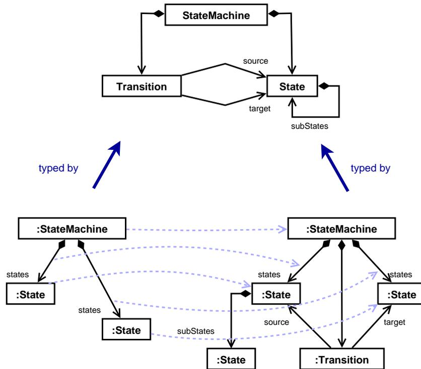
Figure 1: A model graph (top), two instance graphs (bottom) and a typed graph homomorphism.
