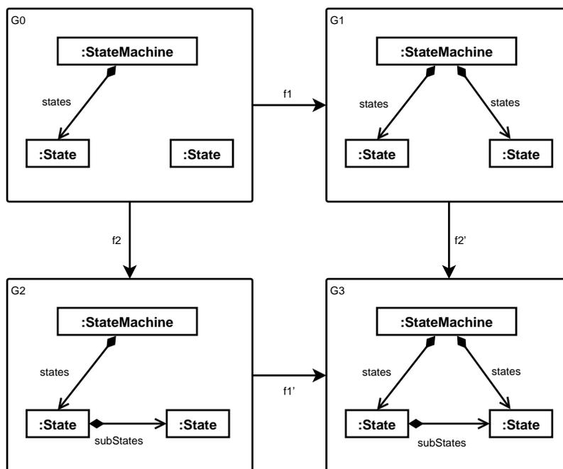
Figure 2: Invalid pushout of graphs with containment edges. A State node in the result graph  $G_3$  has two containers.
