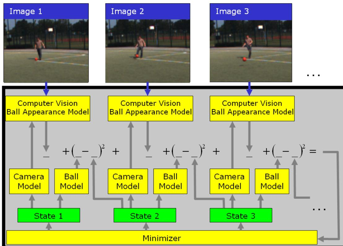
Figure 6: Information flow in a ball tracker based on the global likelihood optimization paradigm (see text). Here, computer vision, i.e. the ball appearance model, is part of the optimization loop (gray box).
