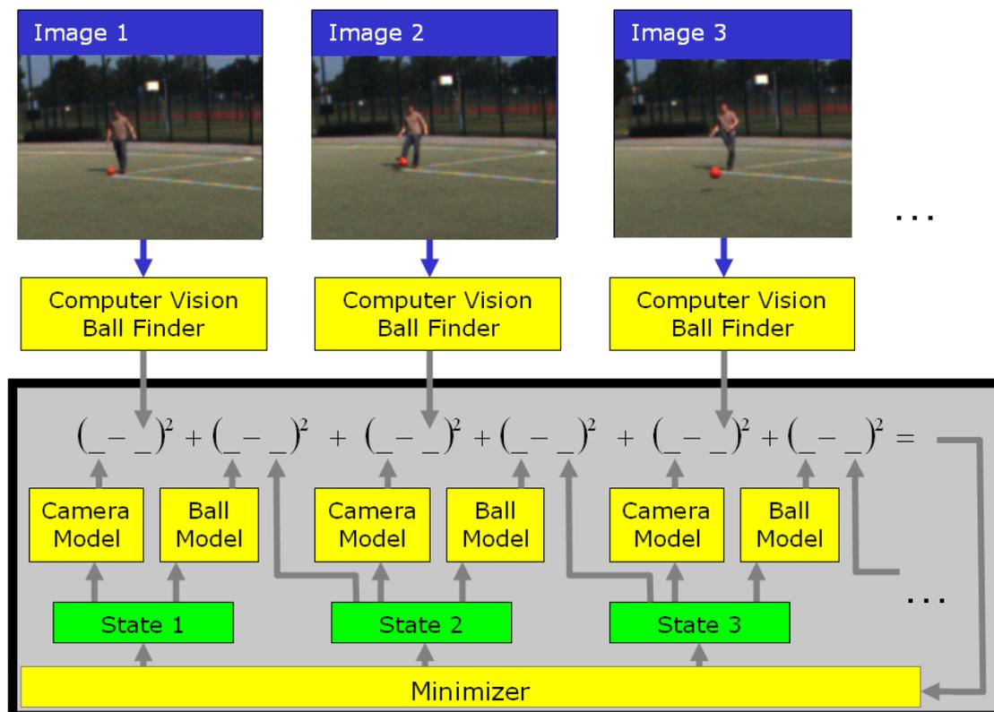
Figure 5: Information flow in a ball tracker based on the conventional data-driven paradigm (see text). The ball finder is not part of the optimization loop (gray box).
