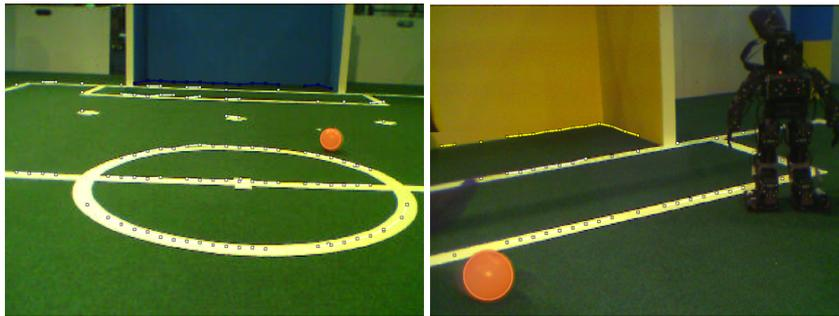
Figure 4: Two images taken and processed by a humanoid soccer robot on a standard RoboCup field [LR07]. The colored dots and lines indicate perceived parts of goals and field lines; the recognized ball is bordered by an orange circle.
