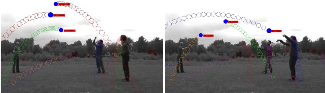
Figure 10: Camera view of the tracking scenario and overlaid detection results (red circles) and predicted ball trajectories (coloured circles).
